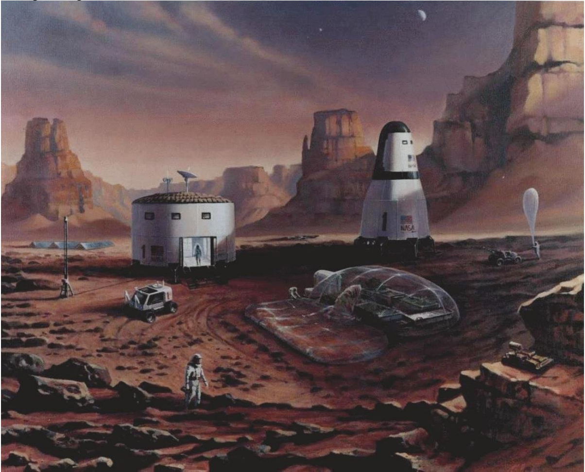
Fig. 1 The Mars Direct plan. First an unfueled Earth Return Vehicle (ERV, right) is delivered to Mars where it manufactures its propellant from the Martian atmosphere. The crew then flies to Mars in the tuna-can-shaped hab module, which also provides living quarters, lab, and workshop for a 1.5 year Mars stay. (Artwork courtesy of Robert Murray, Pioneer Astronautics.)
